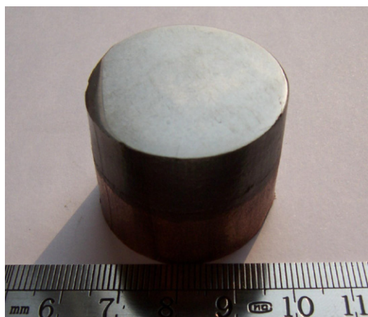
Fig. 2. A W/Cu FGM mock-up made by resistance sintering under ultrahigh pressure.
